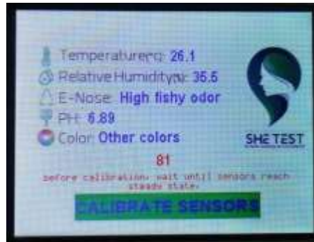
Figure 4: Appeared message on the LCD for calibration
